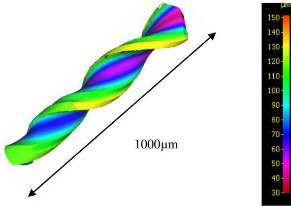
Fig. 6: Measurement of a micro drill bit with Focus-Variation. The colors represent the distances to the axis of the tool.
