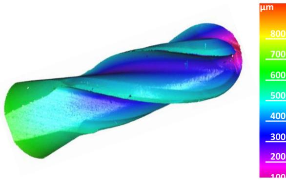
**Fig. 3:** 3D dataset of a measured micro milling cutter. The colors represent the distance to the tool axis.
