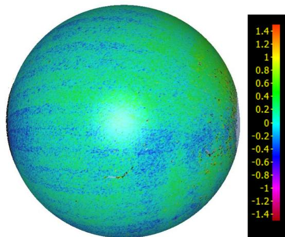
**Fig. 12: Measurement of a calibrated sphere with pseudo colors where the different colors represent the difference of the measurement points to the fitted sphere. The scale is in [ $\mu$ m].**
