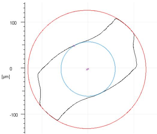
Fig. 7: Measurement of a micro drill bit with major diameter of ~250µm. Extracted contour profile (black) with fitted circles for major (red) and core diameter measurements (blue).
