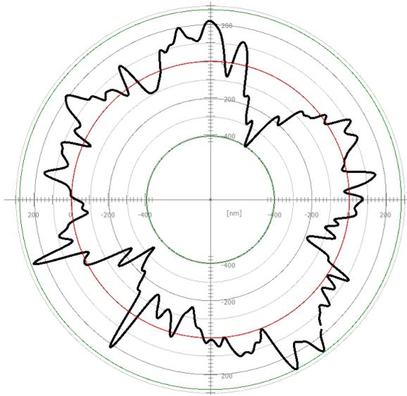
**Fig. 1: Roundness profile generated by a planar cross section through the measured calibration sphere. The deviations to the fitted circle (red) are scaled and lie between -400nm and +250nm**
