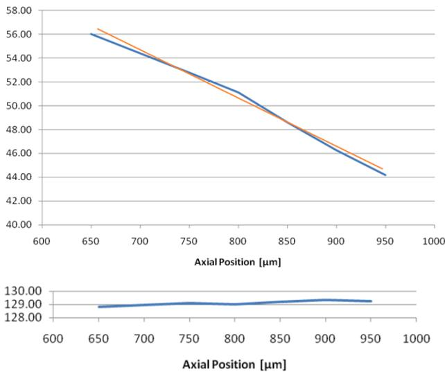
Fig. 8– Upper diagram: Core radius at different axial positions (blue) and fitted regression line (orange). Lower diagram: Major radius at different axial positions.
