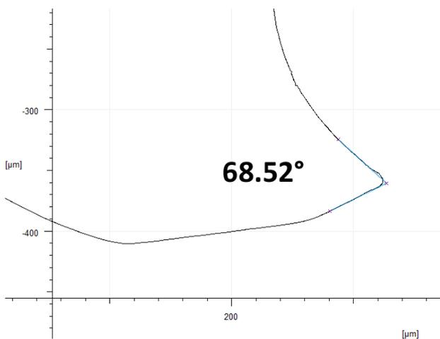
**Fig. 5:** Detailed view of rake angle measurement from the extracted contour. The two lines that have been fitted for angle measurement are shown in blue color.
