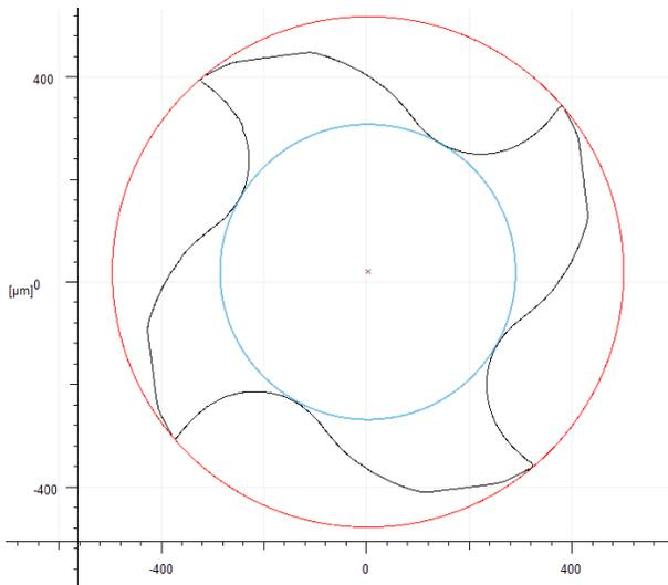
**Fig. 4:** Extracted profile contour of the measured micro milling cutter. Red circle: Outer diameter. Blue circle: Core diameter.
