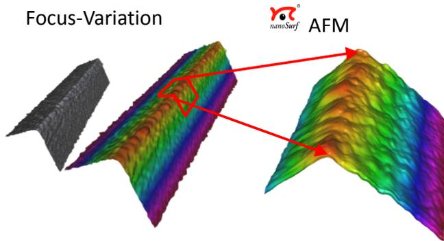
**Fig.9: Comparison of cutting edge radius measurement between Focus-Variation and an atomic force microscope.**
