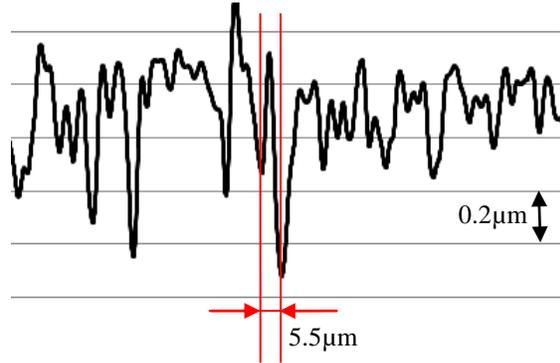
**Fig. 15: Surface detail of the measured roughness profile. The diagram shows that also lateral structures with small wavelengths (<6µm between two valleys in this case) can be measured.**
