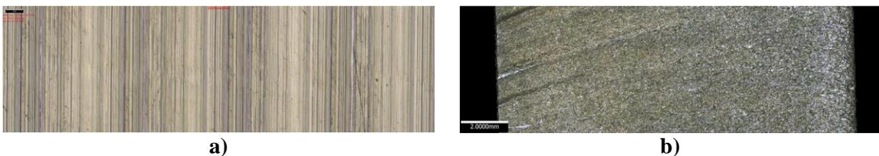
*Fig. 4 Surface morphology: a) after turning, b) after abrasive water jet machining*
