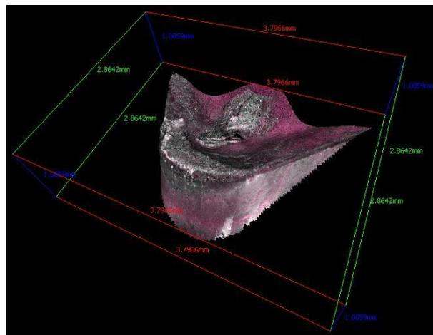
**Fig. 9** Topography of the tool point wear
