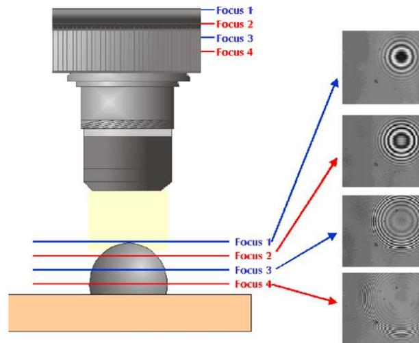
*Fig. 2 Principle of a vertical scanning interferometry [17]*
