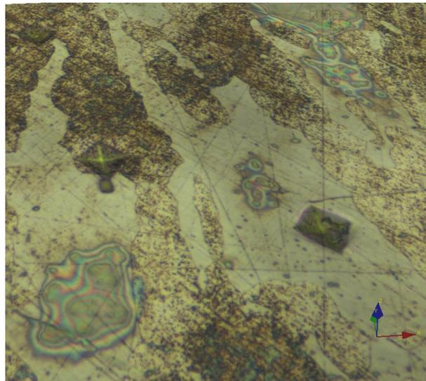
**Fig. 6** Trace the indenter on the surface of duplex steel (dark: ferrite, bright: austenite)
