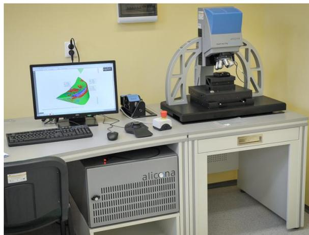
*Fig. 3 Infinite Focus Measurement Machine*
