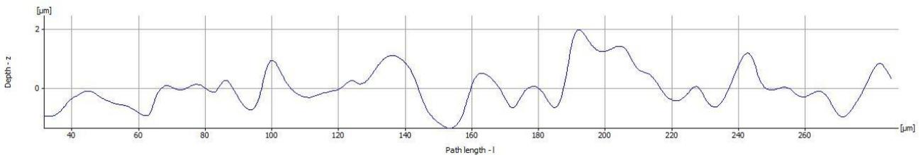
**Fig. 7** Surface roughness profile for Ra parameters- Lc 800 µm
