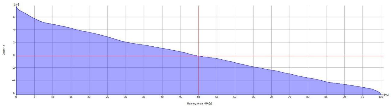
**Fig. 8** Load capacity curve (Firestone-Abbott Curve for Roughness Profile)
